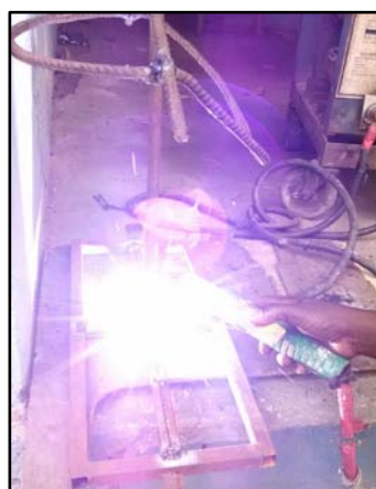
Fig. 35: welding inner to base support
