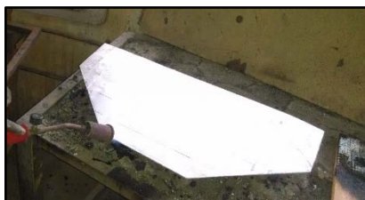
Fig. 18: Annealing Al. sheet for the forming processes
