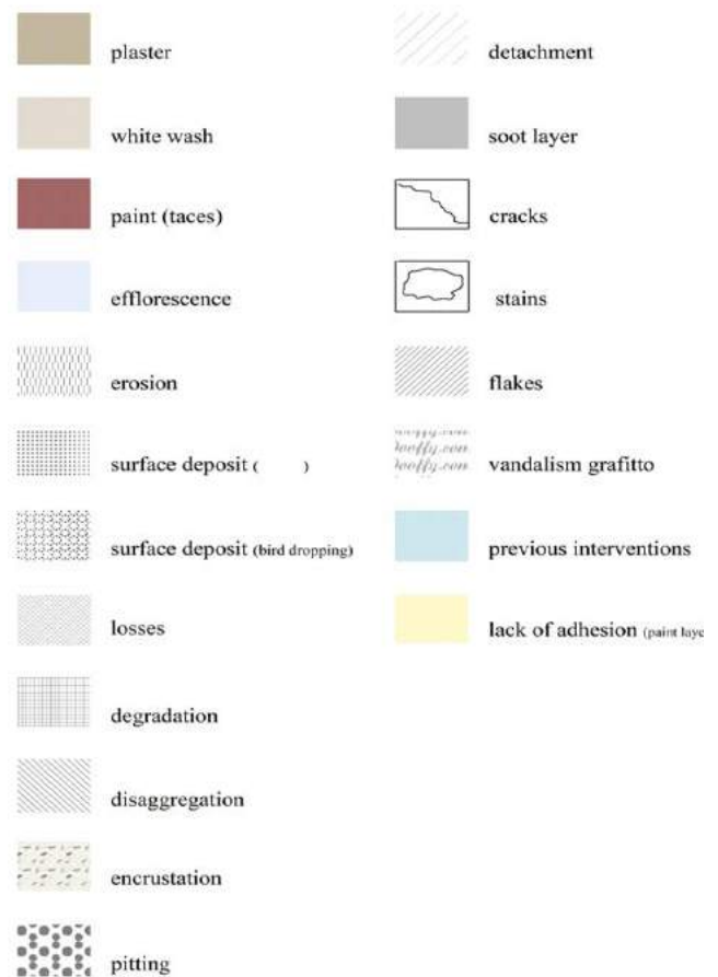
Figure 9: Shows table of types of decay signed in different patterns and colors for documentation as a key to describe the type of damage that exists.
