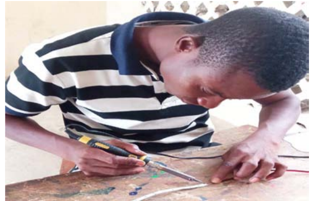
Plate 8: Soldering the LED strip to the wire (Author's fieldwork 2019)
