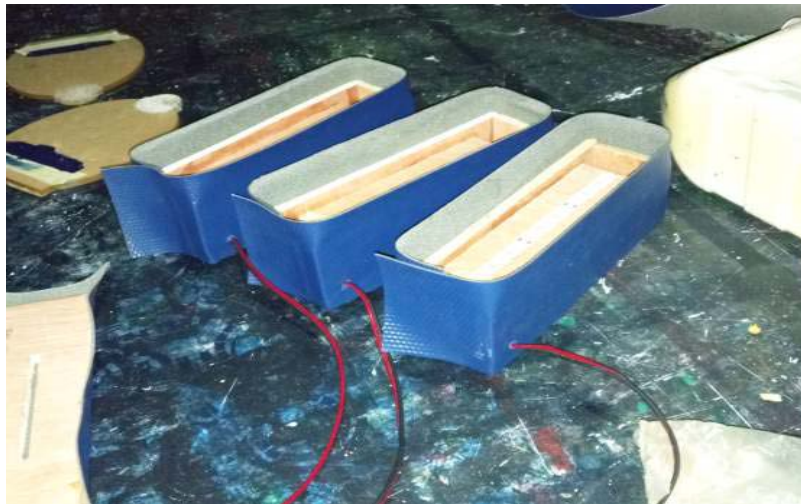
Plate 12: Wrapping lamp casing with leather (Author's Collections, 2019)
