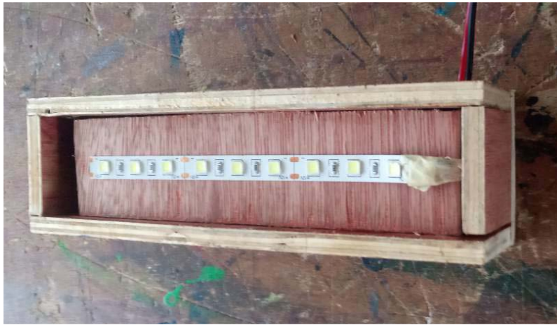
Plate 11: The LED strip being pasted into the base casement (Author's fieldwork 2019)
