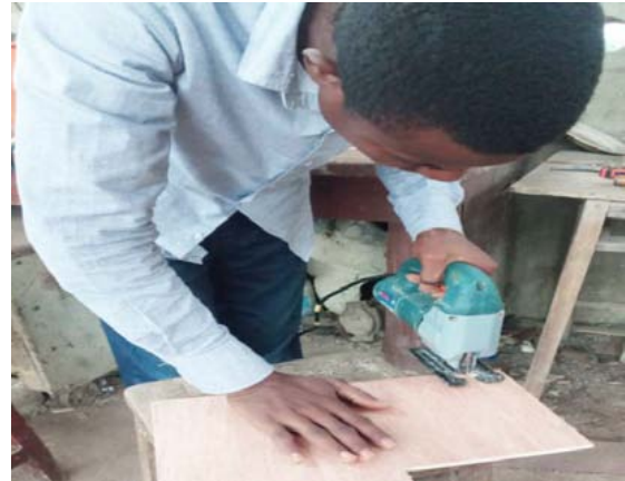
Plate 6: Cutting the plywood with electric jigsaw (Author's fieldwork, 2019)
