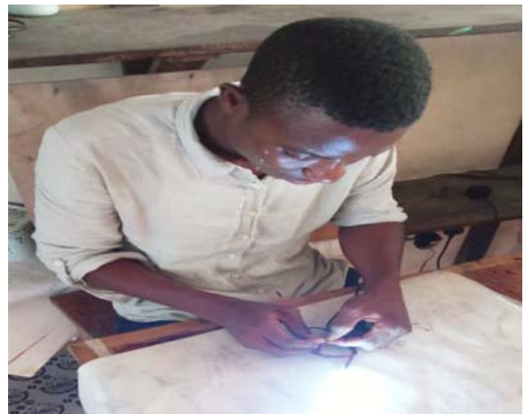
Plate 10: Testing of the LED strips after soldering (Author's fieldwork 2019)
