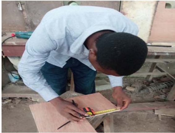
Plate 5: Measuring the plywood to size before cutting (Author's fieldwork, 2019)
